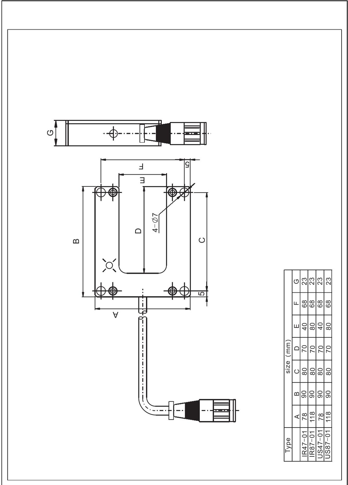
**Appendix III:** Installation drawing for EAGLE EYE I photoelectric sensor
